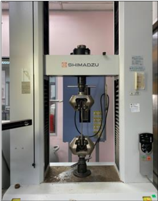
Figure 3. Set-Up for The Pull-Out Test
