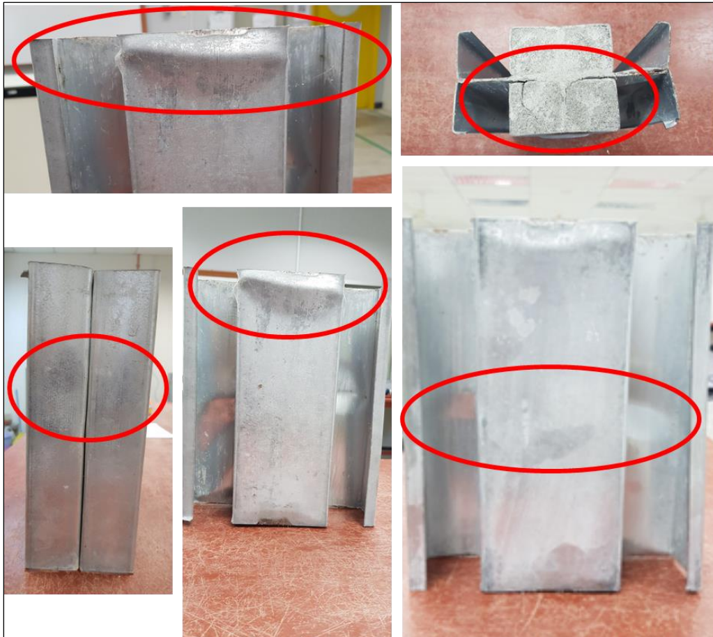
Figure 10. The Failure Mode of The BCFS3 Specimen
