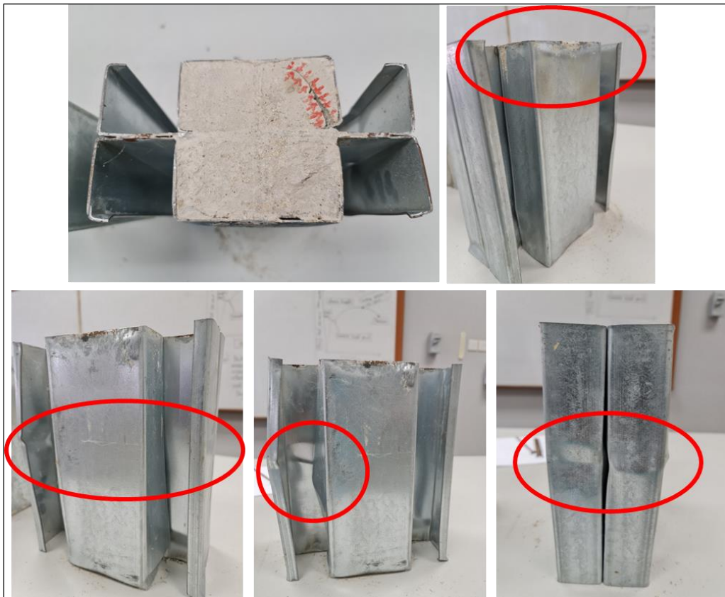
Figure 9. The Failure Mode of The BCFS2 Specimen
