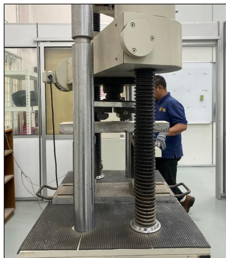
Figure 5. Set-Up for The Flexural Strength Test
